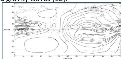
Fig.1: Contours of ionospheric time delay, units of nanoseconds at 1.6 GHz.
